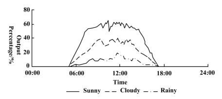
Fig. 2. Output percentage of PV under different weather conditions in summer
