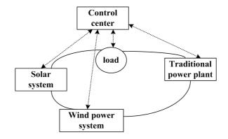
Fig. 1. Typical structure of VPP
